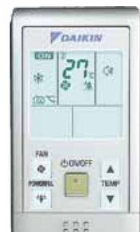
LCD panel with backlight
